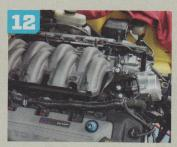
The engine in place—snug as a bug in a rug! Notice that in this shot the Fore fuel rails are installed and the fuel system installation is under way.
