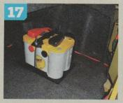
With underhood space at a premium, a new battery tray was sourced from Summit Racing Equipment, and an Optima Yellow-Top battery was placed in the trunk.
