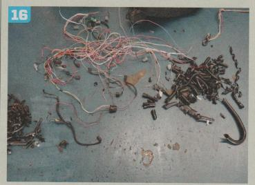
The Pro-Dyno wiring cart got quite a workout during this built. This pile shows the remnants of what was removed from the stock harness. Paul Conner spent many hours to get all of the stock gauges to work, and ended up using an old-school Steeda Timing Adjuster to make the stock tachometer interface with the new engine computer—a use we're sure the Steeda engineers never intended.
