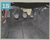
Because the Coyote uses a drive-by-wire throttle arrangement, the use of a new throttle pedal assembly was required, along with come custom wiring to get everything to communicate correctly.
