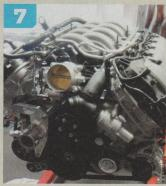
Another view of the completed Vintage Air kit installed on the front of the engine, with the power steering pump in place.
