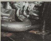
With the use of the Vintage Air kit, the air conditioning compressor and powersteering pump required custom lines to be made at a hydraulics specialty shop to match up with the New Edge's factory components on the other end.
