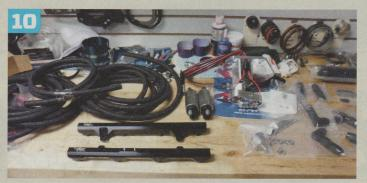
A complete fuel system from the experts at Fore Innovations was employed to provide the New Edge Coyote with the correct fuel volume. Fore Innovations even engraved the Pro-Dyno logo atop the new rails! The system arrived with all new hose, one of Fore's awesome dual-pump fuel hats, a pair of Walbro GSS342 pumps, filters, a 0 to 100-psi fuel pressure gauge, and all of the fittings and fasteners required for installation.
