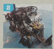
The easiest way to take out the factory engine (provided you have a lift) is to just disconnect the transmission, suspension, exhaust, and harnesses, and then drop it right out the bottom of the car with the springs and struts still attached. As none of these pieces were reused, it made the task a quick one.
