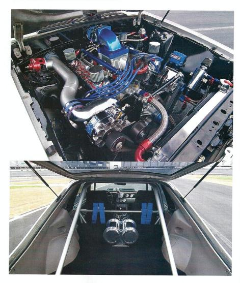
through a K&N filter in the cowl vent just below the windshield. An elbow-shaped Wilson upper manifold mates to an Edelbrock Super Victor intake plenum. Eight Lucas high-impedance injectors can flow up to 72 pounds of fuel per hour with the help of a Barry Grant fuel pump and regulator.
