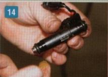
14. Paul applies a thin film of lube to the bottom of each injector. This keeps the O-ring seal from tearing itself up during installation.
