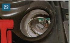
22. Don't try to move this lock ring with your bare hands! A light mallet or hammer, a notched screwdriver and some finesse are required. Notice the non-threaded outlet on top of the factory pump; some welding will give us a much sturdier -6 AN connector once the unit is away from the car and has dried.
