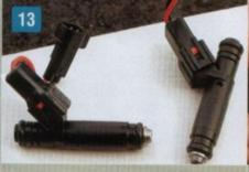
13. These 60lb injectors should keep the blown 4.6 fed well above 5,000 rpm; stock units are 24-pounders. This kit came with wiring adaptor clips (shown) for a Ford application.
