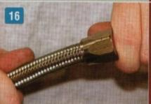
16. Because he is performing the fuel system upgrade from scratch, Paul must cut and fit his lines after careful measuring. These braided lines will be used in the hot engine compartment.
