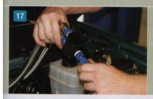
17. After installation, a bracket will be made to mount the Y-block, but for now the three hoses keep it securely in place.
