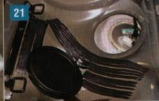
21. On the driver's side of the transmission tunnel, prying off the rubber cap gives access to the top of the standard fuel pump.
