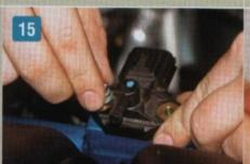
15. The fuel rail pressure sensor (FRPS) will be relocated to the center of the new rail. Adjusting the wiring harness to reach it only required cutting, then re-taping, the protective wrap. There was no cutting or splicing of wires necessary.
